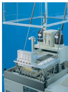
Picture of the Chemspeed system used and the 2 mL small scale reactor
