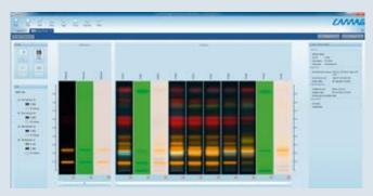
"Comparison Viewer": Selected tracks of images taken from different plates under UV 254 nm, white light and UV 366 nm can be displayed side by side.
