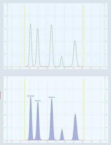
Automatic baseline correction and peak integration of six different sulfonamides
