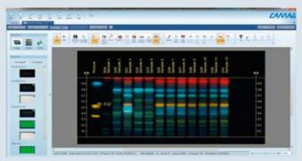
**"Data View"** allows for visual evaluation of a plate in different illumination modes and offers a broad range of helpful tools, *e.g.* a  $R_{\rm F}$  tool displays the  $R_{\rm F}$  value of zones on the digital image or a rectangular zoom function.
