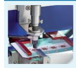
The extraction efficiency and analysis quality is ensured via the application of an internal standard prior to the extraction. The internal standard solution is applied with a high a precision sprayer onto the DBS. CAMAG has been manufacturing high precision application instruments for HPTLC for a long time and has used this experience to build this module.
