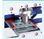
The extraction unit seals the DBS card and solvent is guided horizontally through the DBS into a sample loop. The loop volume can be of various sizes and configurations according to the application. The extract is guided online to the analysis system and is independent from the extraction solvent cycle.
