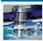
A designated wash station cleans all parts that are in contact with the DBS cards and additionally flushes the entire tubing to avoid any carry-over. Using this system, independent user tests confirm that carry-over is not an issue.
