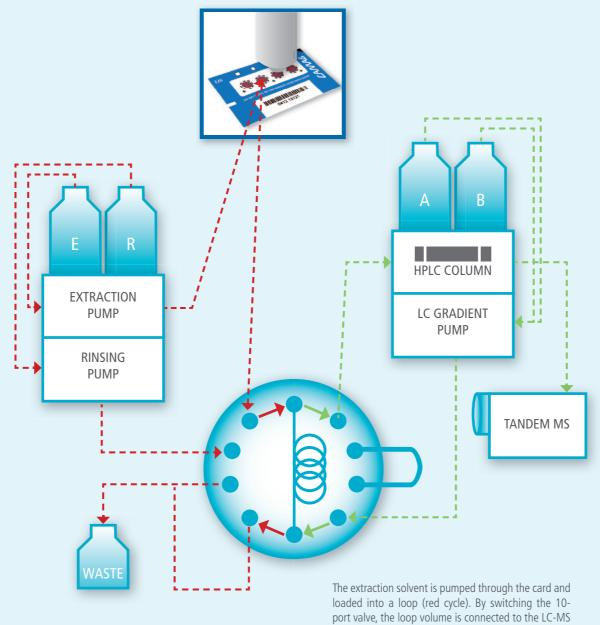
flow path (green cycle) and guided to the column and after separation to the tandem MS. Meanwhile, the extraction head is cleaned by a rinsing cycle to avoid
