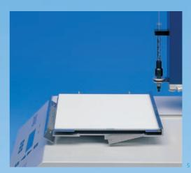
The self-adjusting object support enables application onto objects of variable thickness (up to 4 mm) without any adjustment to the spray nozzle. This makes changing between conventional TLC and HPTLC layers, on glass plates and sheets, preparative layers and very thin objects such as membranes easy. The support accommodates objects up to 20×20 cm.
