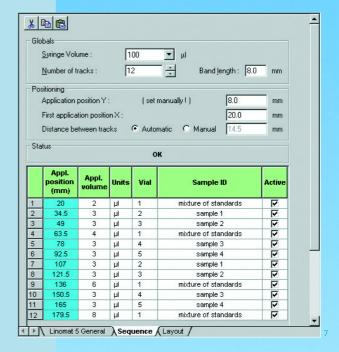
The system proposes a corresponding layout. Before sample application begins the user is prompted to confirm that the syringe contains the correct sample.
