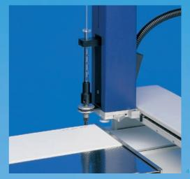
The sample liquid is sprayed onto the layer from the tip of the syringe needle.
