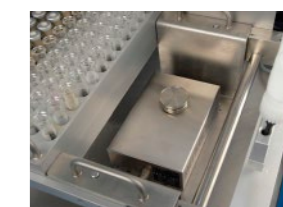
Integrated balance module for gravimetric dispensing of e.g. butadiene
